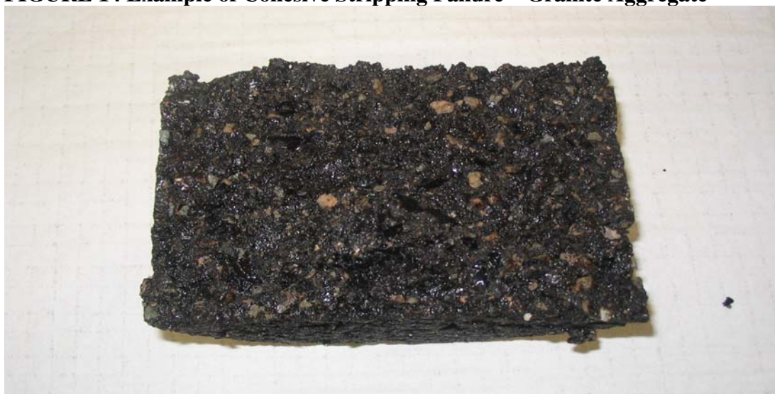
FIGURE 15 Example of Adhesive Stripping Failure – Granite Aggregate
