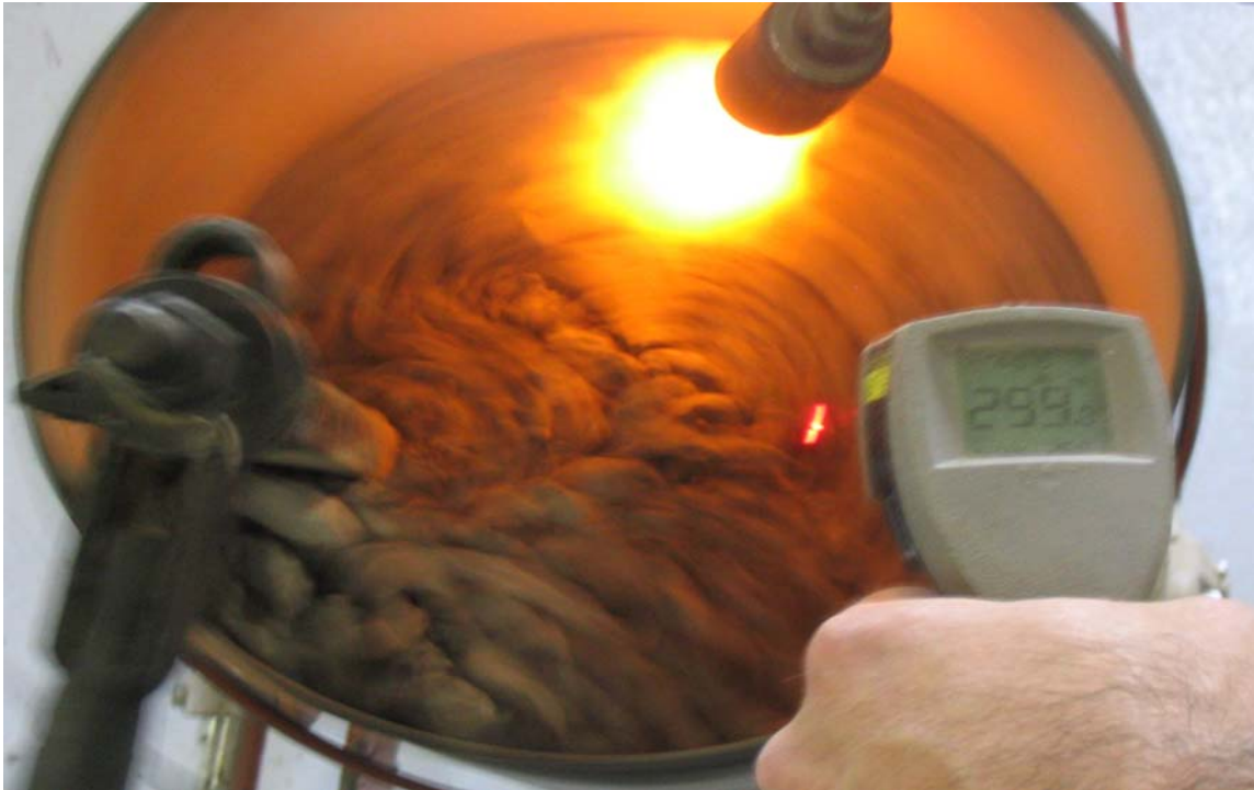
FIGURE 3 Heating of Wet Aggregate to Mixing Temperature
