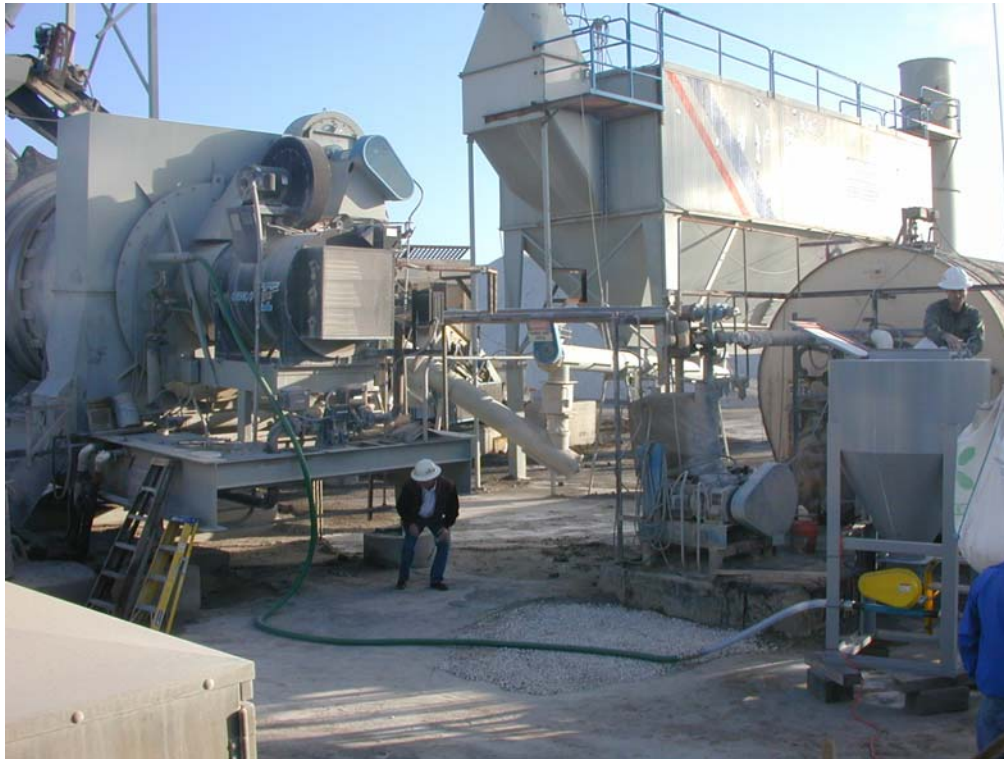
FIGURE 16 Feeder for Aspha-min® Zeolite
