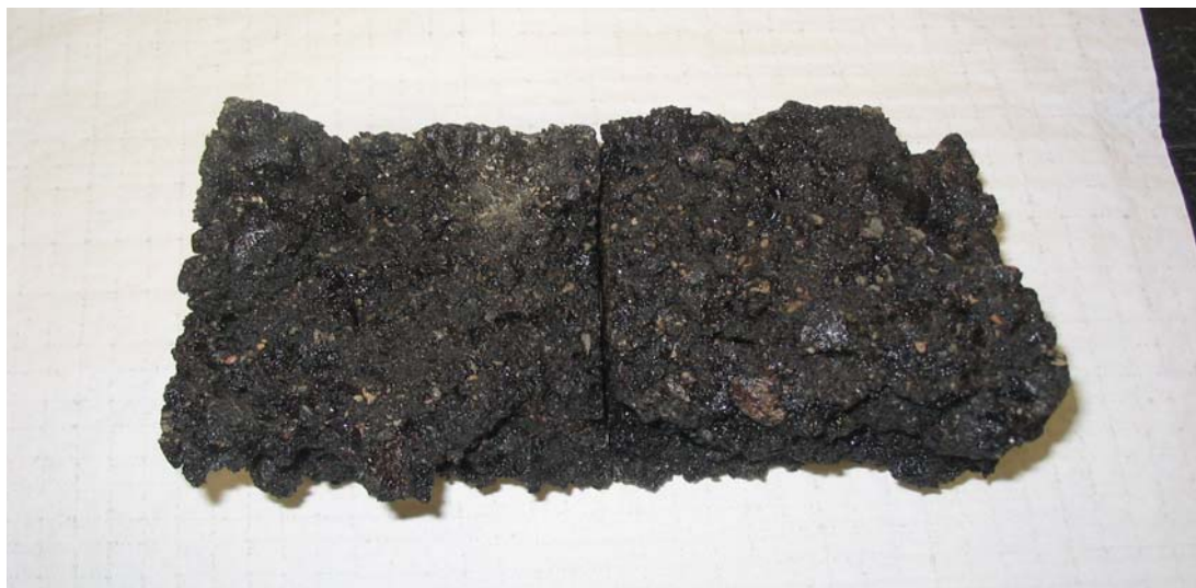
FIGURE 14 Example of Cohesive Stripping Failure – Granite Aggregate
