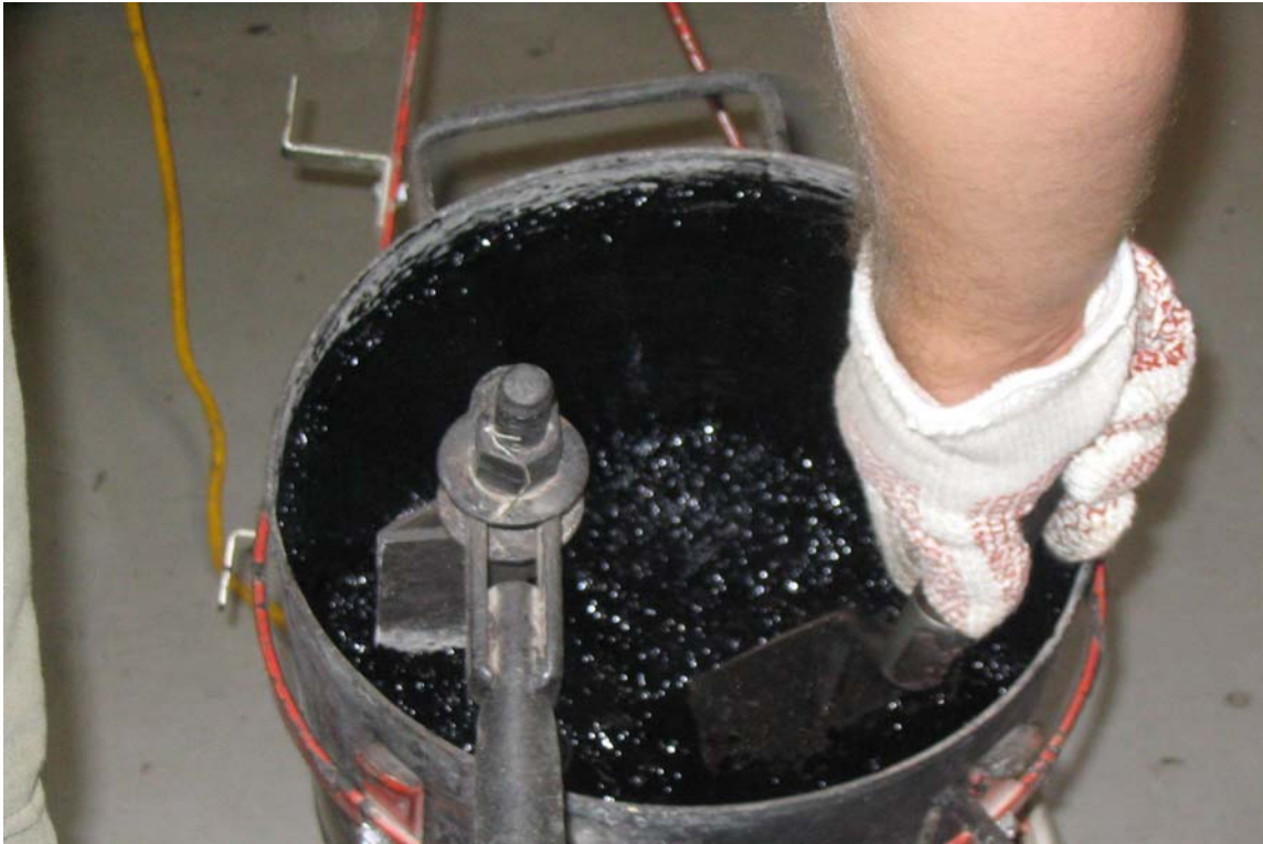
FIGURE 4 Hot Mix Asphalt in Bucket Mixer
