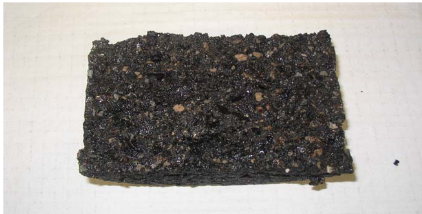
Figure 15. Example of Adhesive Stripping Failure – Granite
