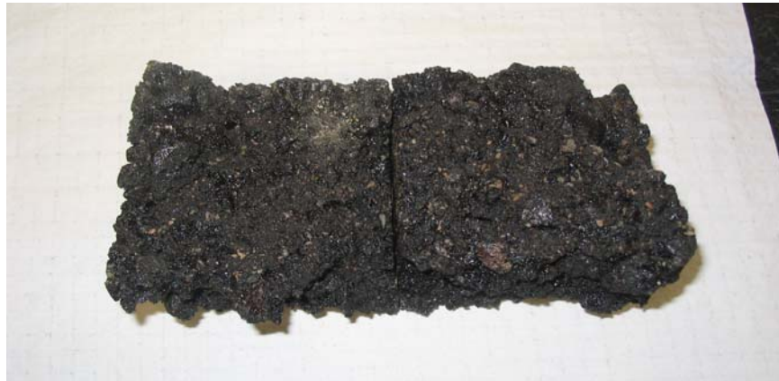
Figure 14. Example of Cohesive Stripping Failure – Granite
