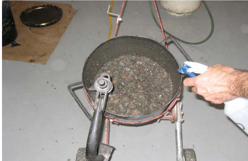
Figure 2. Introduction of Moisture to Aggregate for TSR Samples
