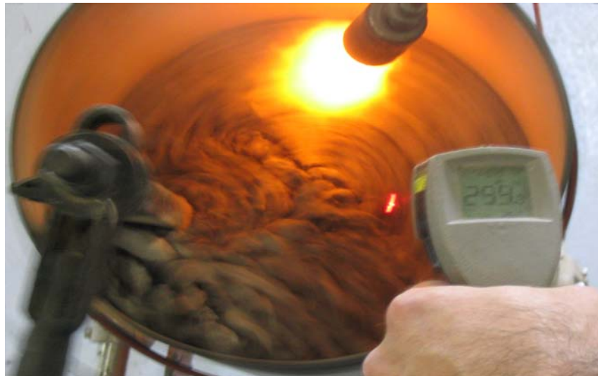
Figure 3. Heating of Wet Aggregate to Mixing Temperature
