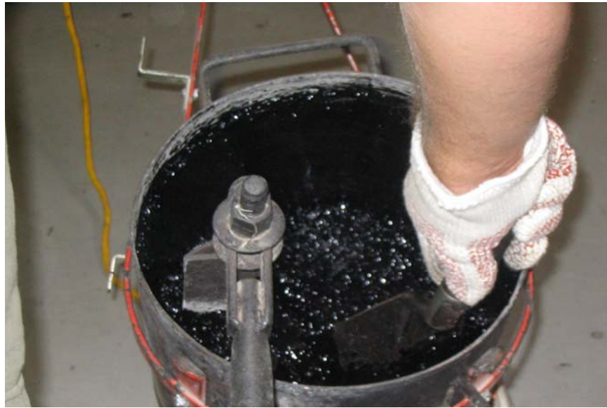
Figure 4. Warm Mix Asphalt in Bucket Mixer
